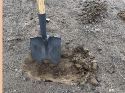
Typical tailings. Depending on level of oxidation, unoxidized tailings can also exhibit metallic luster from the arsenopyrite present. Shovel for scale.
