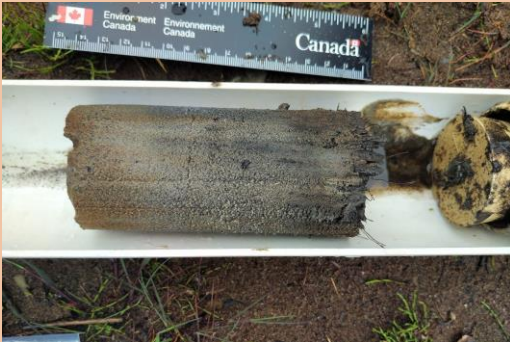
Sediment core of tailings from an impacted wetland. The grey color at the top of the core (right hand side) indicates the presence of unoxidized tailings, while the lower part of the core is more rusty in colour.
