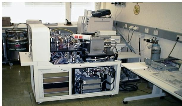
*Figure 3. Laser based system for breath test analysis.*
