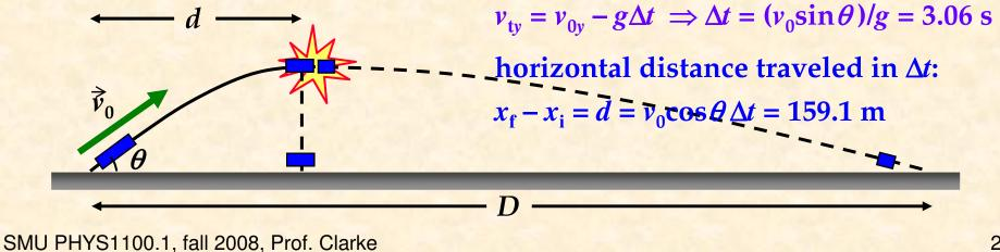
2. At the top, we conserve momentum immediately before and after the explosion. Let  $m_1 = \frac{2}{3}m$  be the larger mass that drops to the ground, and let  $m_2 = \frac{1}{3}m$  be the smaller mass that is propelled forward. Then,
