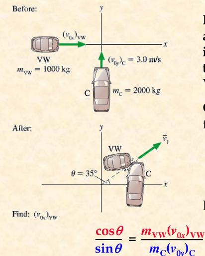
In a car accident between a Cadillac (C) and a Volkswagen (VW), the two cars interlock bumpers and stay together after the collision. What was the velocity of the VW just before impact?
