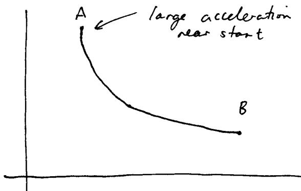
A cycloid corresponds to the locus of a point on the circumference of a circle rotating along a fixed line.
