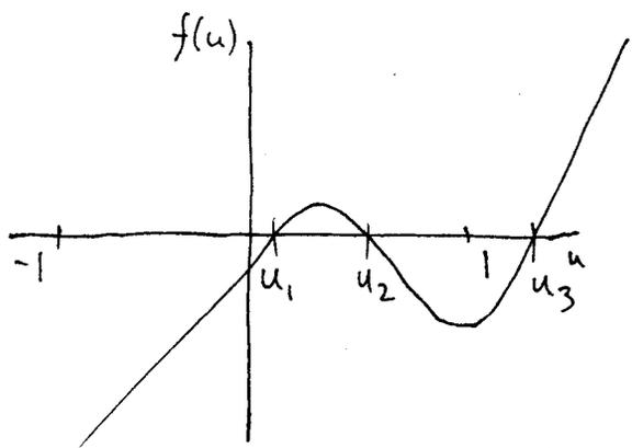
for the top on the plane we expect two solutions with  $u > 0$  (but this need not be the case if the top was supported on a tall pivot)
