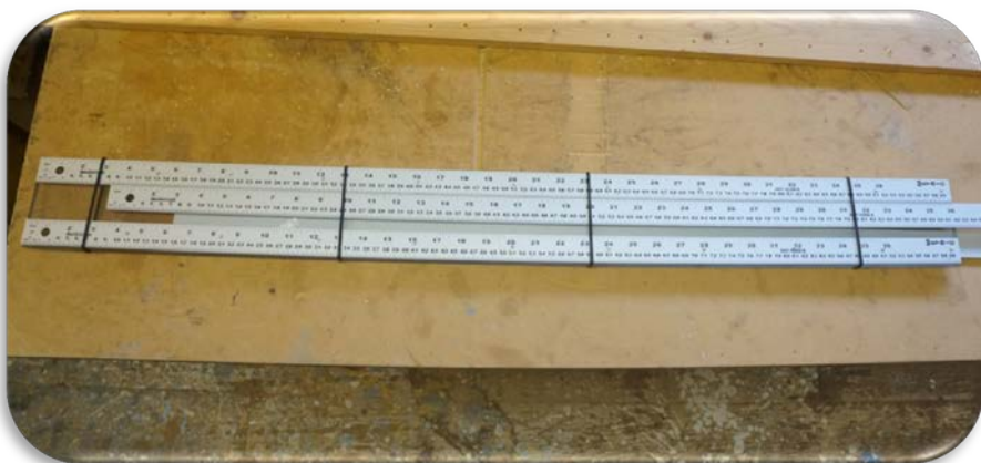
4. Slide four o-rings over the board, spacing them out evenly.
