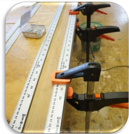
3. Secure rivets with rivet gun. Repeat steps 1-3 with second metre stick (running in same direction). Sand rough edges.
