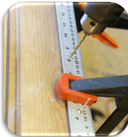
2. Drill 10 holes through metre stick and plastic board. Insert rivets as holes are drilled to prevent metre stick from sliding during drilling.
