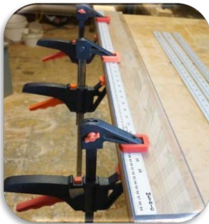
1. Align a metre stick along edge of plastic board and clamp in place. Place a board behind the plastic to prevent cracking during drilling.
