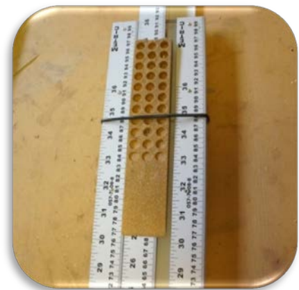
6. Slide levelling wedge under the top-most o-ring to provide tension for front sliding ruler.
