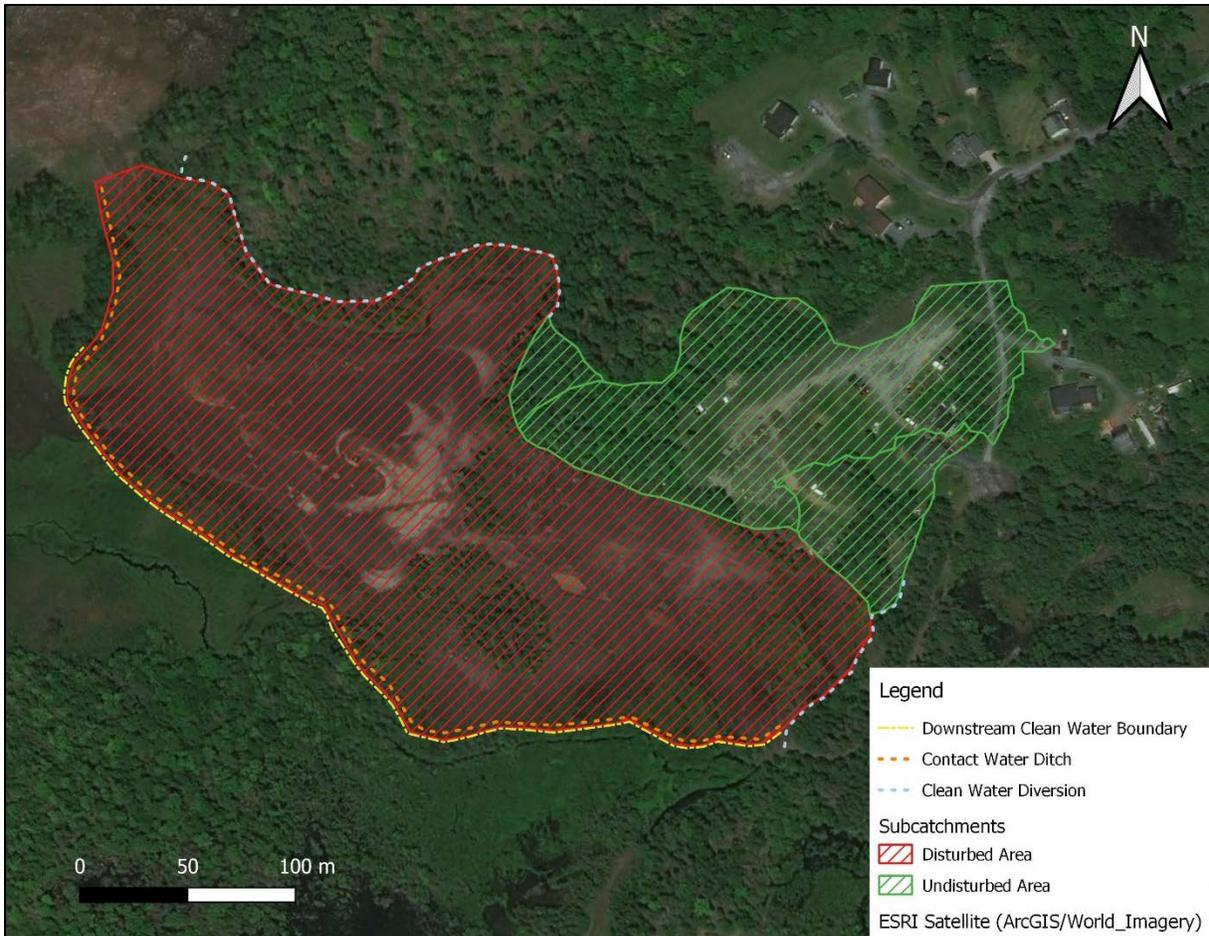
**Figure 1. Montague Conceptual Water Management Strategy during Construction**
