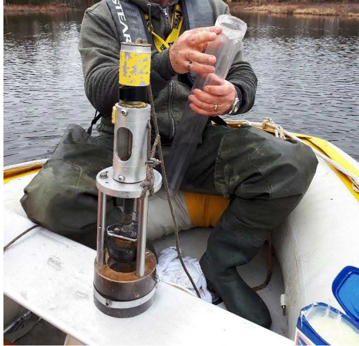
Photo 15. Glew Gravity Corer used for the sediment sampling program (April 16, 2019).
