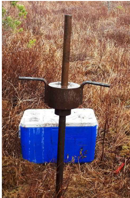
Photo 18. Manual split spoon used to collect soil samples (April 25, 2019).
