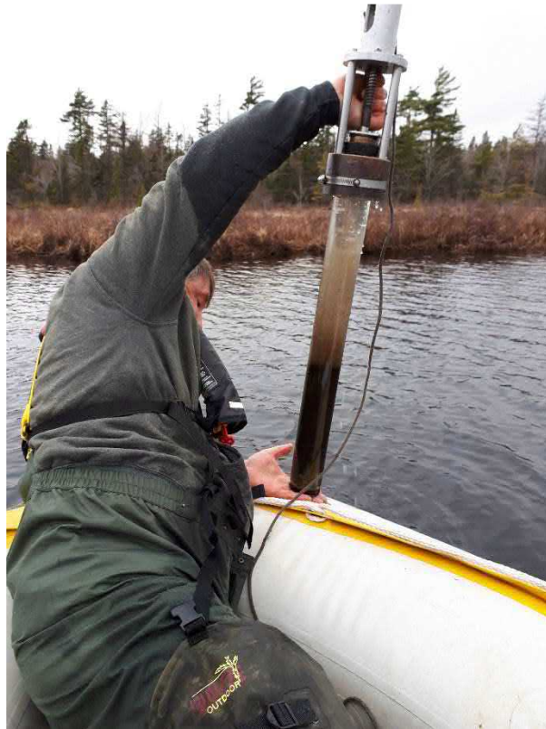
Photo 16. Glew Gravity Corer used for the sediment sampling program (April 16, 2019).
