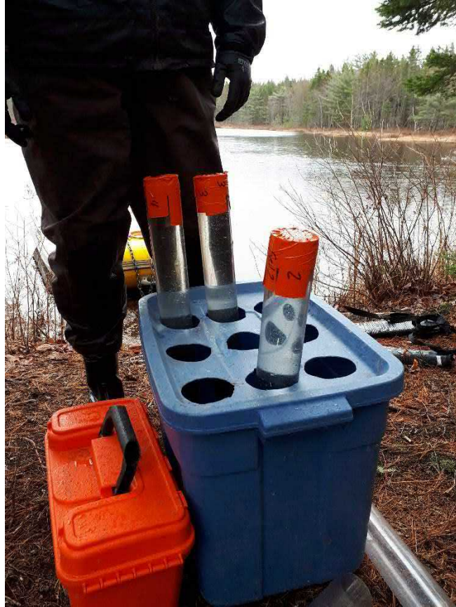
Photo 17. Sediment cores collected using the Glew Gravity Corer (April 16, 2019).
