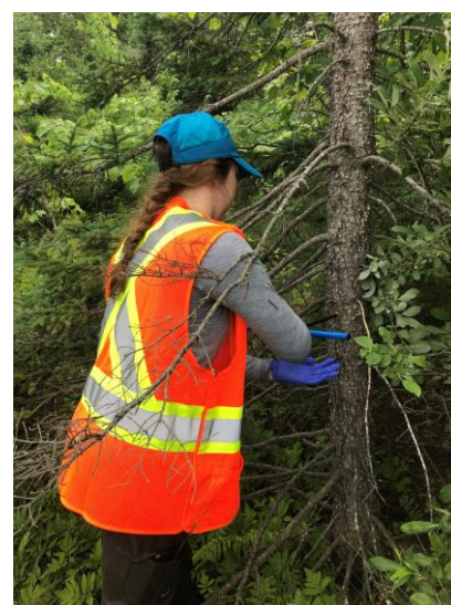
Me, taking a core sample from a Spruce tree at a mine tailing site
