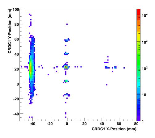
Figure 2.4: CRDC 1 y-vs-x spectrum with a mask placed in front of the detector.
