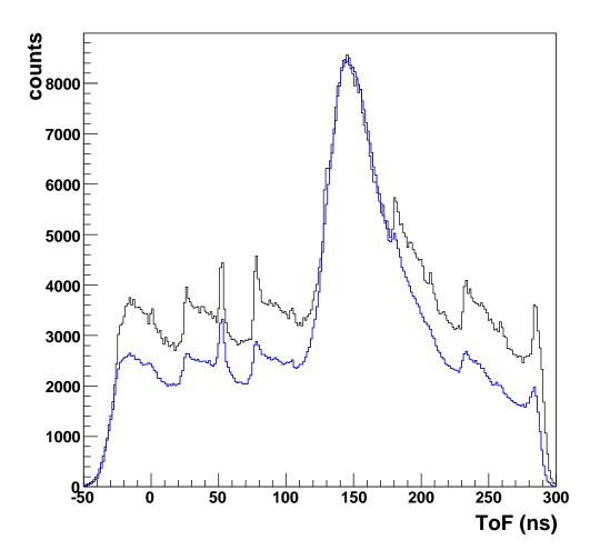
Figure 5.1: Neutron ToF for normal (blue) and high rate (black) runs.
