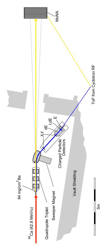
Figure 2.2: Experimental setup.
