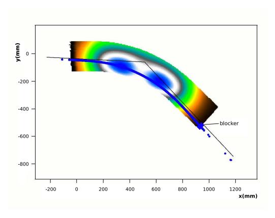
Figure 3.8: Track of a 2.8 Tm particle through the magnetic field of the sweeper. The blue curve is the path of the 2.8 Tm particle, while the black line represents the central trajectory. The location of the tungsten blocker is indicated on the figure.
