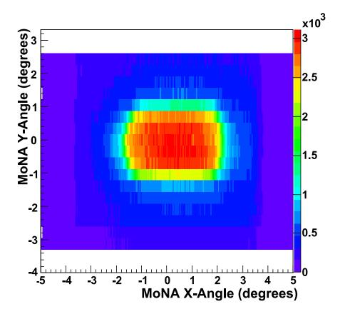
Figure 2.6: Plot of MoNA y-angle vs. x-angle, demonstrating the limited acceptance caused by the quadrupole tiplet.
