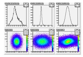
(a) Example two-dimensional ROOT histogram displaying b1p0Ekin vs. b2p0Ekin, with user defined binning of 300 bins between 400 and 800 on the x-axis and 300 bins between 2960 and 3070 on the y-axis.
