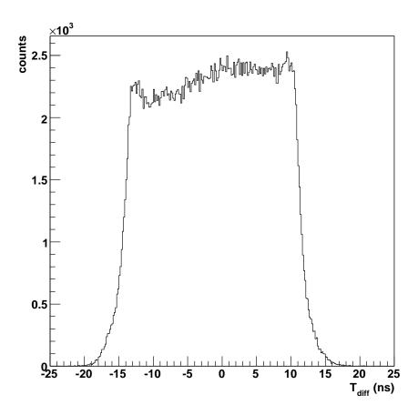
Figure 2.5: Time difference spectrum for the center bar in MoNA's front layer.
