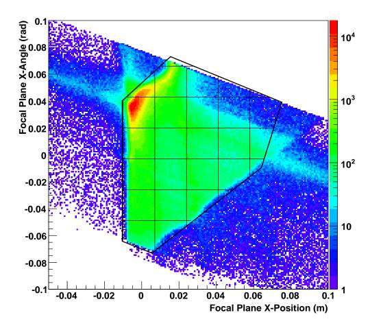
Figure 3.2: Focal plane angle vs. position. The black outline indicates events which are accepted for analysis, and the inner lines are the boundaries of the grids used for calculating ToF corrections. The peak around  $\theta_x \simeq 0.04 \, \mathrm{rad}$ ,  $x \simeq 0.005 \, \mathrm{m}$  is composed primarily of scattered background events, which are excluded as described in section 3.2.
