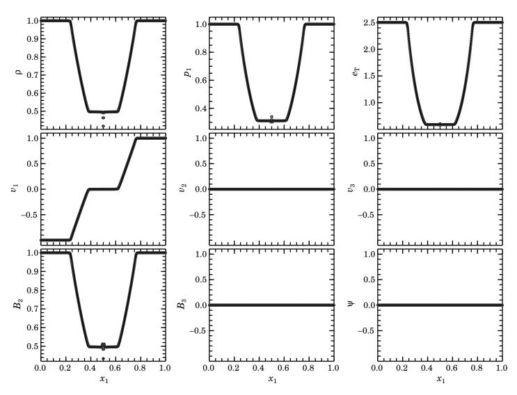
This is Fig. 3b from Ryu & Jones (1995, ApJ, 442, 228), showing the solution of the MHD shock tube problem with the left state  $(\rho, v_1, v_2, v_3, B_2, B_3, p_1) = [1, -1, 0, 0, 1, 0, 1]$  and the right state [1, 1, 0, 0, 1, 0, 1]with  $B_1 = 0$  and  $\gamma = 5/3$  at time t = 0.1. At t = 0, the discontinuity is at  $x_1 = 0.5$ . Plots show from left to right two oppositely-moving magneto-acoustical  $(B_1 = 0)$  rarefactions.
