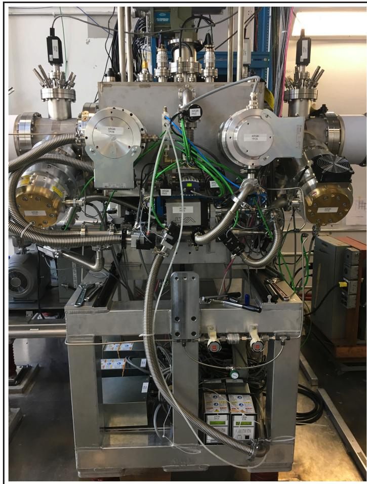
A Radio-Frequency Quadrupole beam cooler and buncher from the charge breeding component of CANREB located at TRIUMF (see abstract by S. Roy-Garand)
