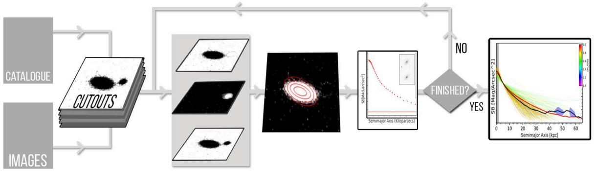
Visual depiction of a surface brightness profile generation program, starting with a catalogue of objects and a set of images to individual surface brightness profiles and further analysis (H. Souchereau)
