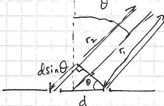
Two slits are the sources of spherical wavefronts
