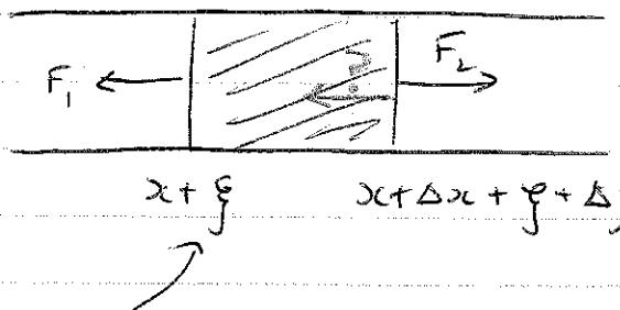
Piece of material of fixed mass is displaced via displacement field
