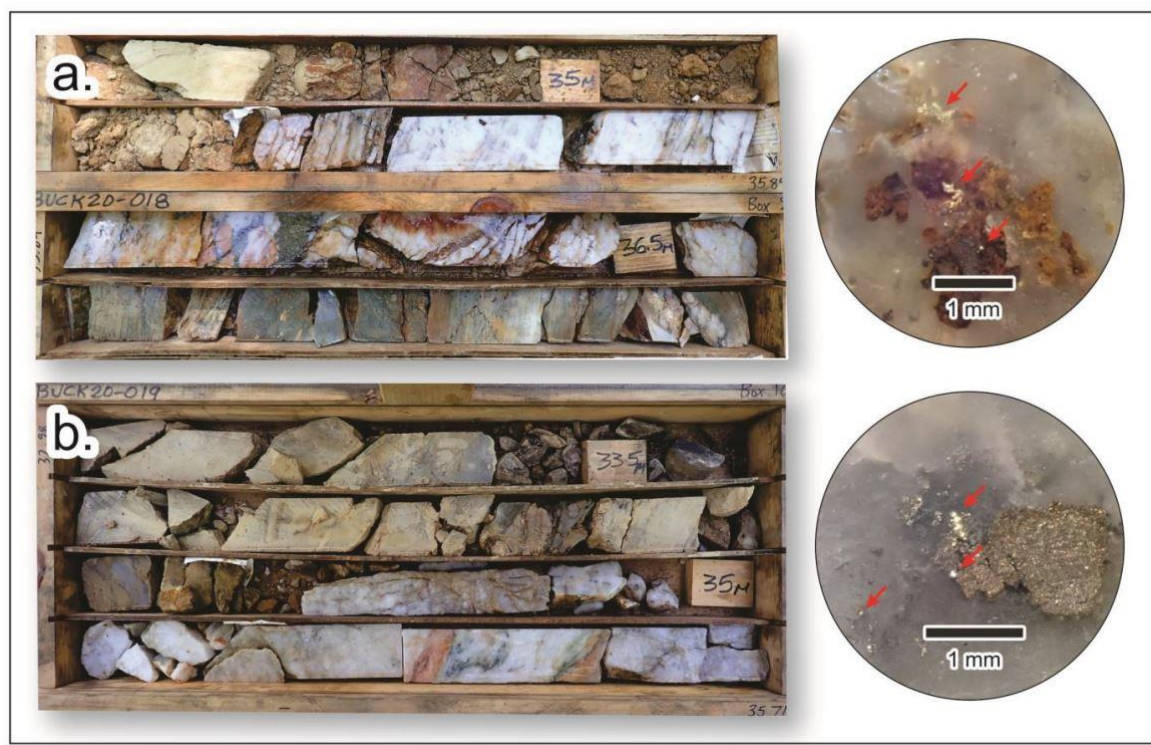
Figure 11: Quartz Vein Intervals – BUCK-018 (a) and BUCK-019 (b) - Red Arrows are Visible Gold
