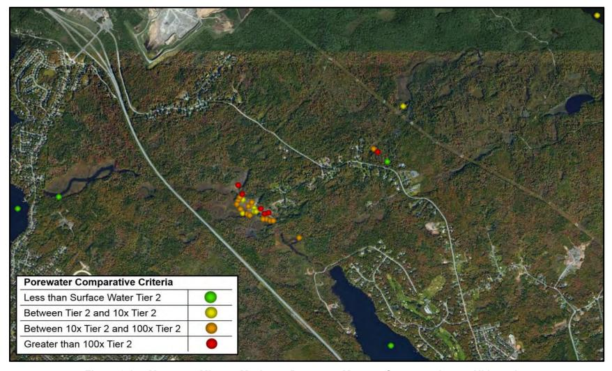
Figure 6-15: Montague Mines – Maximum Porewater Mercury Concentrations – All Locations
