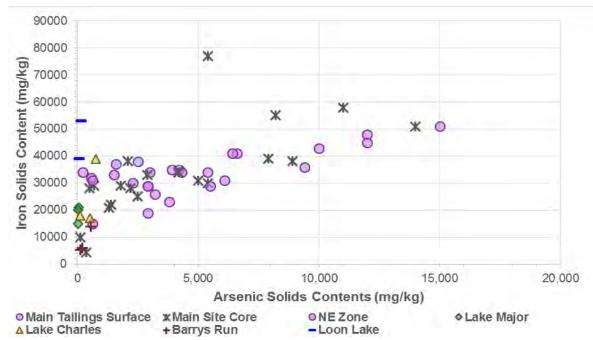
Figure 4-2: Montague Gold Mines – Iron vs. Arsenic Contents in Tailings and Sediments
