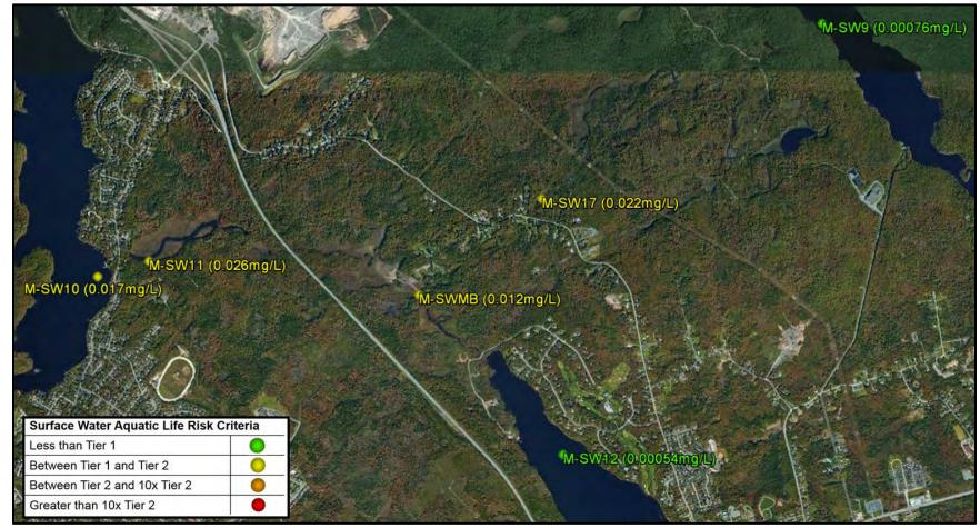
Figure 6-11: Montague Mines – Surface Water Total Arsenic Concentrations
