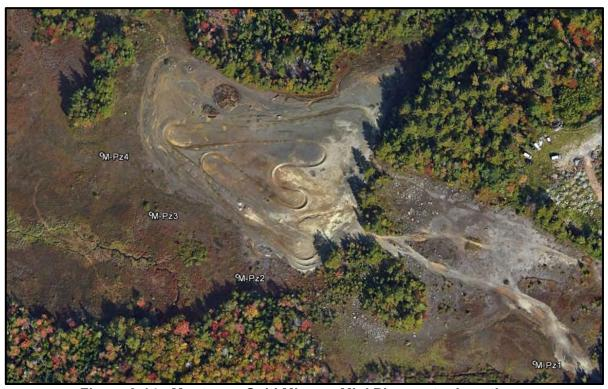
Figure 3-14: Montague Gold Mines - Mini Piezometer Locations
