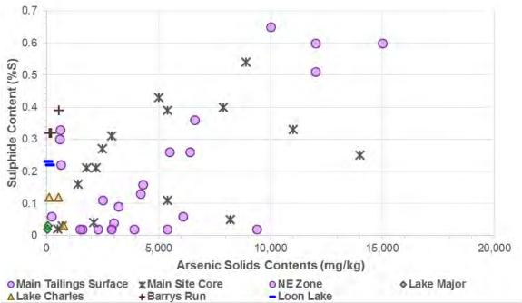
Figure 4-1: Montague Gold Mines – Sulphide vs. Arsenic Contents in Tailings and Sediments
