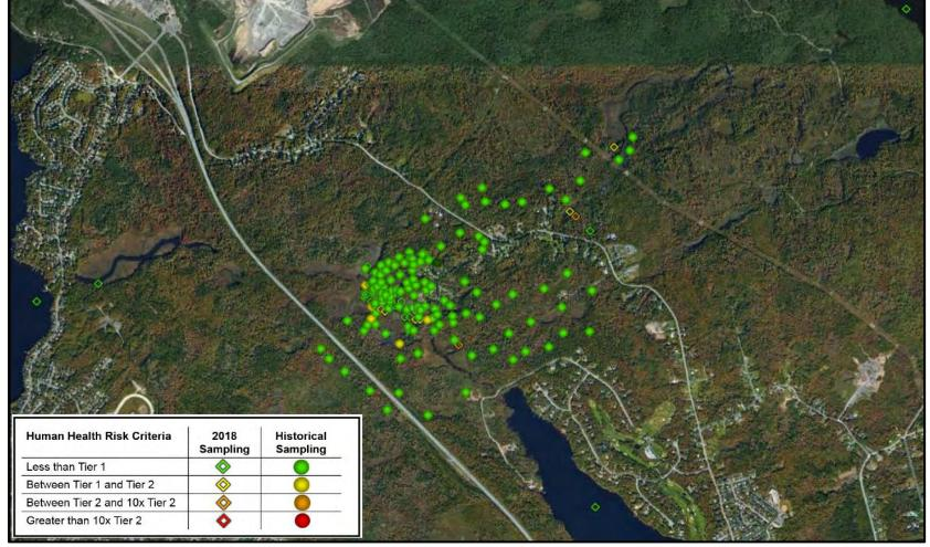
Figure 6-9: Montague Mines - Near-Surface Mercury Contents - All Locations
