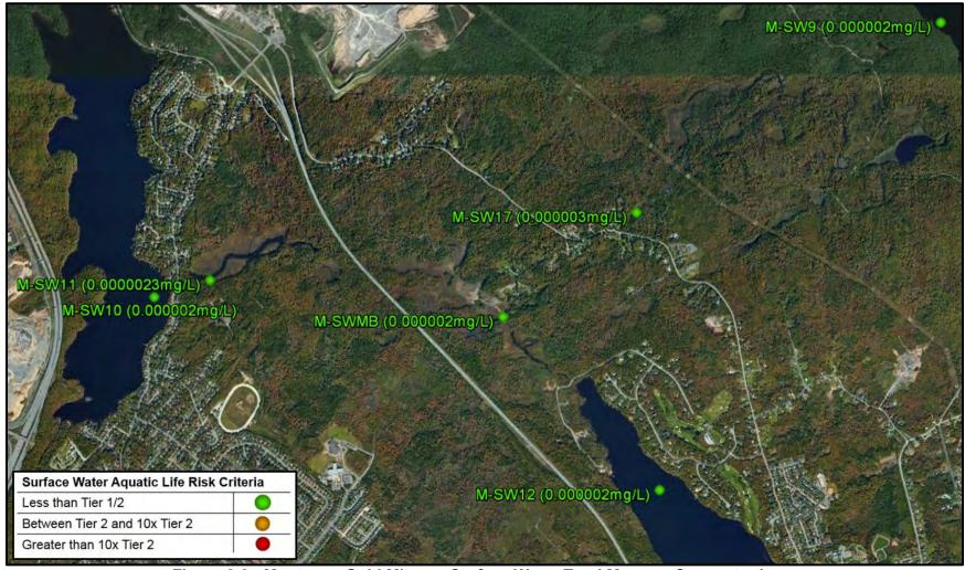
Figure 3-9: Montague Gold Mines - Surface Water Total Mercury Concentrations
