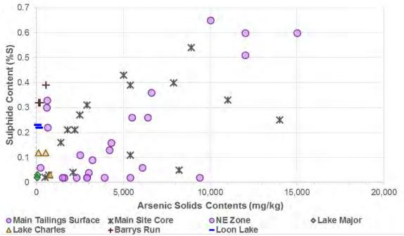
Figure 6-22: Montague Mines - Sulphide vs. Arsenic Contents in Tailings and Sediments
