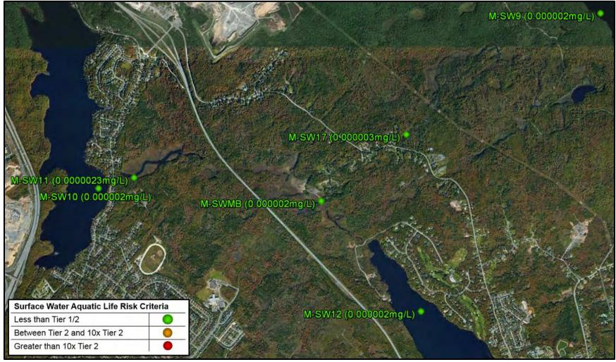
Figure 6-12: Montague Mines – Surface Water Total Mercury Concentrations
