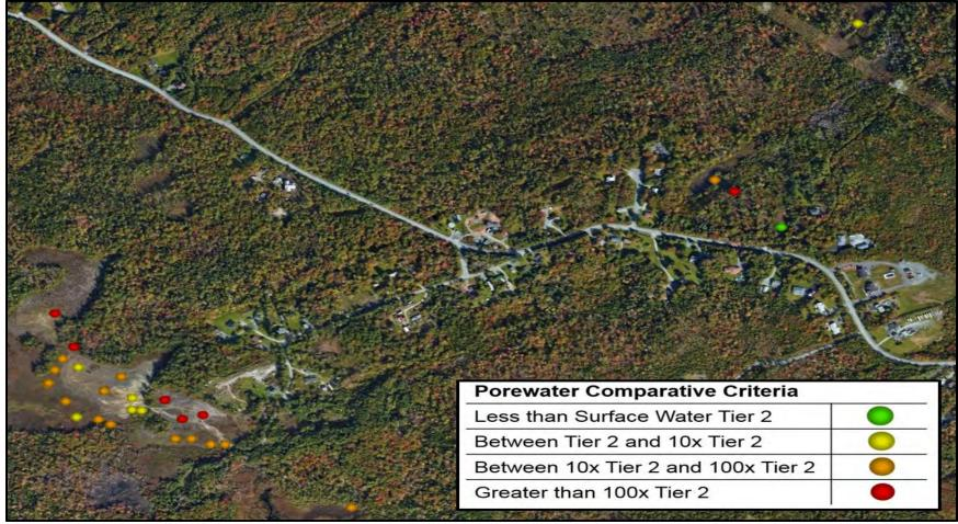
Figure 6-16: Montague Mines – Maximum Porewater Mercury Concentrations - Central Region
