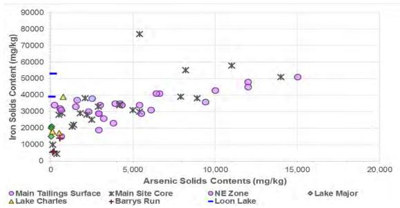
Figure 6-23: Montague Mines – Iron vs. Arsenic Contents in Tailings and Sediments
