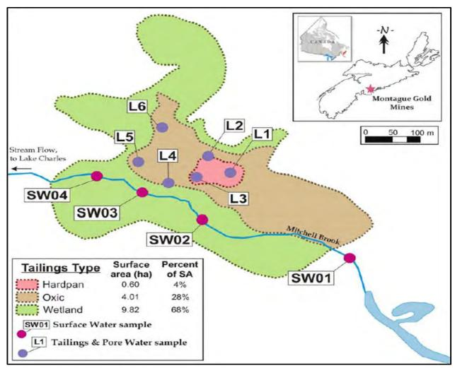
Figure 6-3: Montague Mines – Distribution of Near-Surface Tailings Types at Montague (DeSisto 2014)
