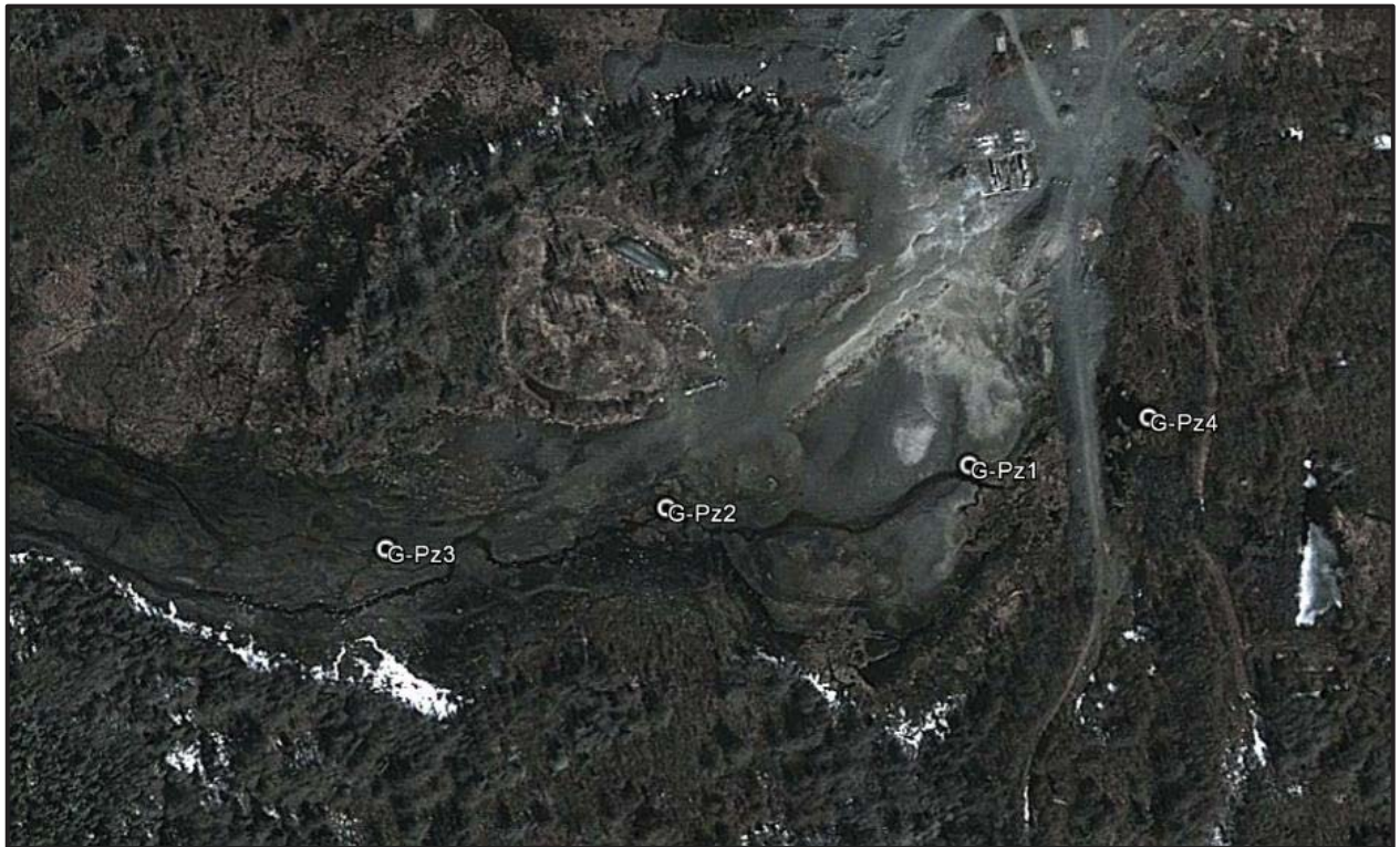
Figure 6-20: Goldenville Mines – Mini Piezometer Locations
