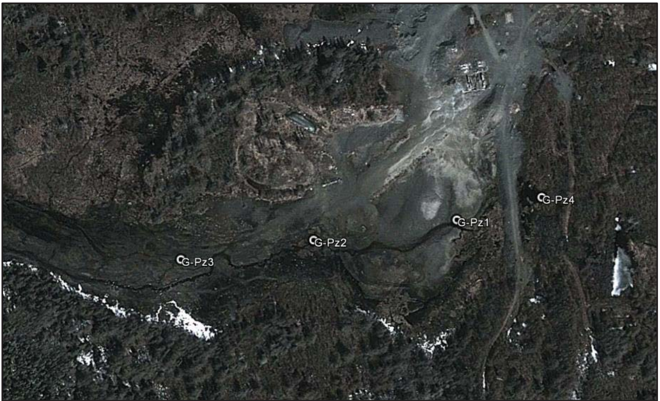
Figure 3-12: Goldenville Tailings Areas – Mini Piezometer Locations
