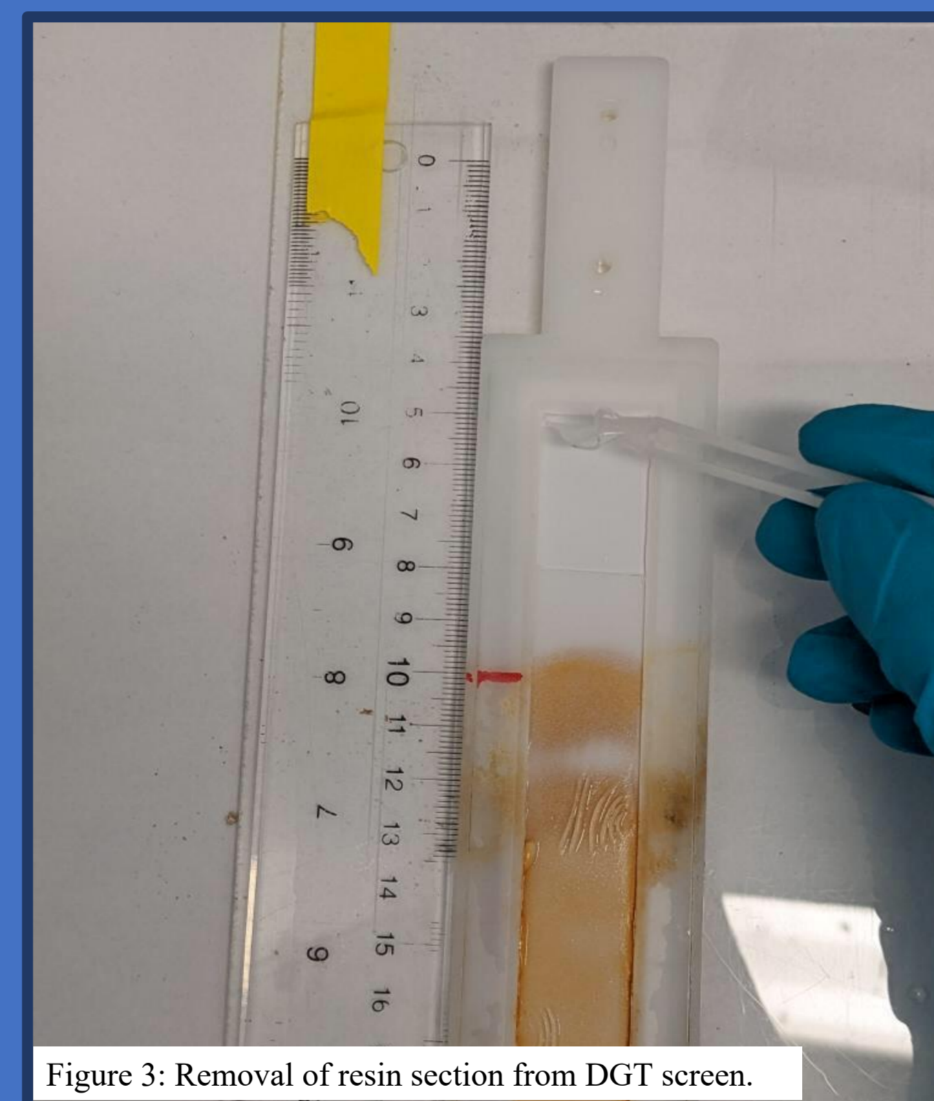
Figure 3: Removal of resin section from DGT screen.
