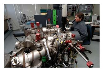
SIMS can perform elemental analysis of sub-ppm concentrations and can achieve per mil precision in <sup>18</sup>O analysis. The big advantage of the SIMS system is the spatial resolution both horizontally and with sample depth. This is obviously dependent on the model but resolutions of 0.12  $\mu$ m are achievable.
