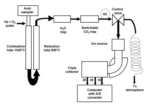
Figure 6. Schematic of the isotope ratio mass spectrometer.
