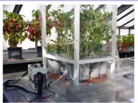
Labelling in the field is possible if the chamber has a suitable flange that allows for the chamber to be driven in to the soil by about 10 cm.
