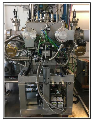
A Radio-Frequency Quadrupole beam cooler and buncher from the charge breeding component of CANREB located at TRIUMF (see abstract by S. Roy-Garand)
